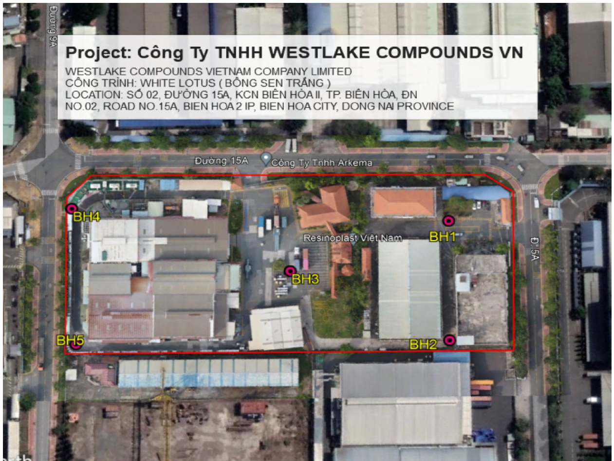
Figure: Locations of borehole
